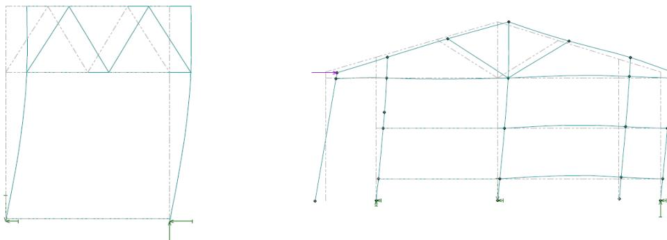
**Figure 1.3 – Deflected Shape of Lateral System**
